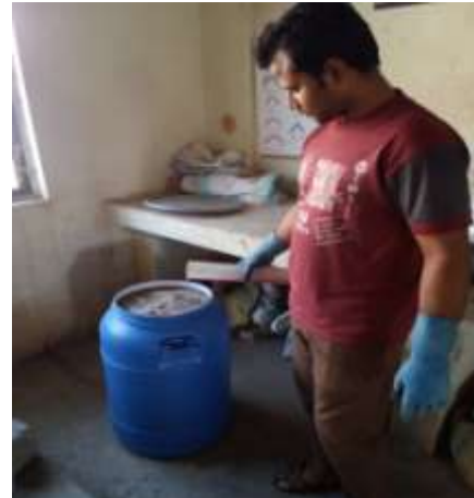
Figure 4 curing of cube specimens in acid solution
