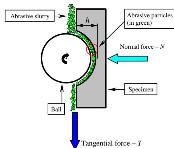
**Figure 1:** Micro-abrasive wear test by rotating ball: a representative figure showing the operating principle and the abrasive particles between the ball and the specimen. “ $h$ ” is the depth of the wear crater.
