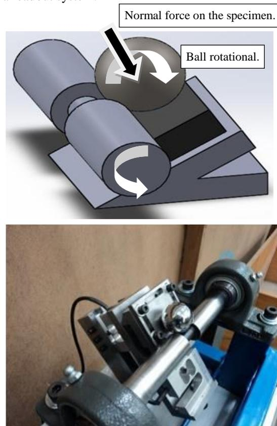
**Figure 3:** Ball-cratering micro-abrasive wear test equipment used in this work: free-ball mechanical configuration, able to acquire, simultaneously, the “*normal force* –  $N$ ” and the “*tangential force* –  $T$ ”.
