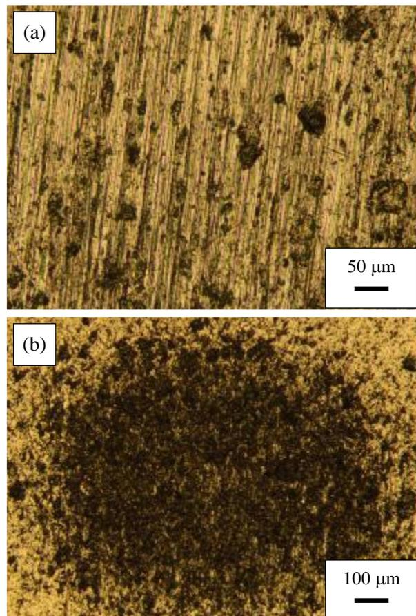
**Figure 5:** Occurrence of (a) “grooving abrasion” and (b) “rolling abrasion” on the surface of the TiN thin film.
