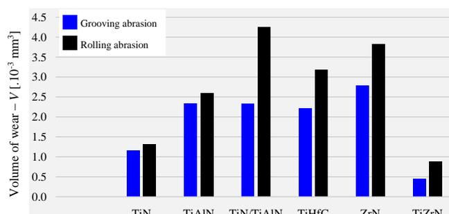
**Figure 6:** Volume of wear ( $V$ ) as a function of the micro-abrasive wear modes. Maximum error of  $V$ :  $3.54 \times 10^{-3} \text{ mm}^3$ .
