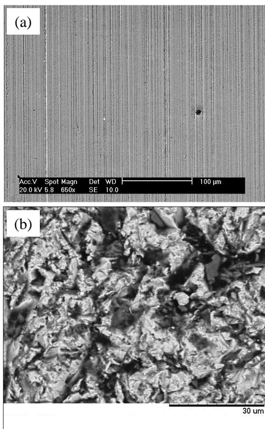
**Figure 2:** Micro-abrasive wear modes: (a) “*grooving abrasion*” [11] and (b) “*rolling abrasion*”.
