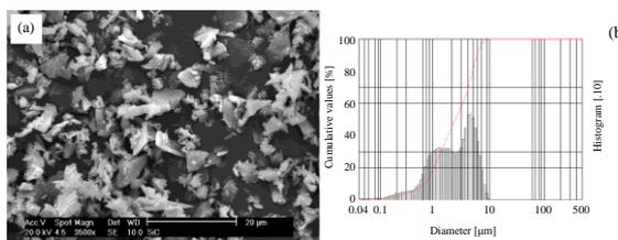
**Figure 4:** SiC abrasive [4]: (a) scanning electron micrograph and (b) particle size distribution.
