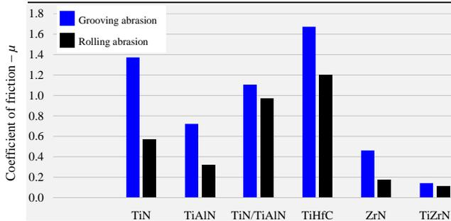
**Figure 7:** Coefficient of friction ( $\mu$ ) as a function of the micro-abrasive wear modes. Maximum error of  $\mu$ : 0.11.
