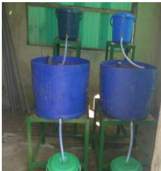
Figure 2: Installation of Lysimeter
