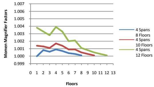
From the above results, it can be seen after conducting a P-Delta analysis of the structure that is reviewed with varying spans and heights to obtain the amplification factor, the final moment, and deflection due to the P-Delta effect. The deflection value and the last moment are more significant than the first moment, so it needs to be controlled against the deflection, and the moment that occurs.
