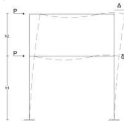
**Picture.** Story Drift and Drift on the portal
