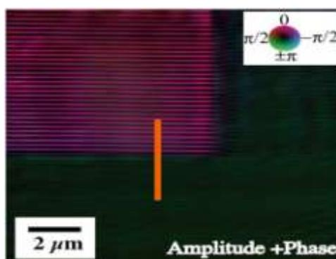
Figure 7. Complex amplitude images of a corner part of  $88\ \text{nm}$  L/S. The amplitude represented by brightness and the phase represented by hue pattern. Reproduced from [10]. Copyright ©2013 The Japan Society of Applied Physics. All rights reserved.
