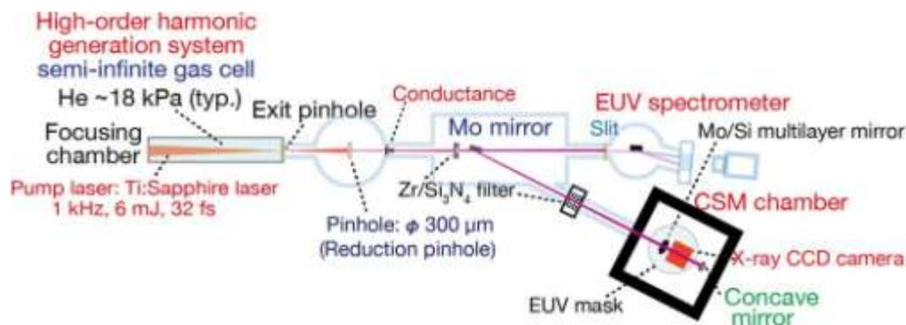
Figure 13. Upgraded optical relay for the HHG-CSM system.
