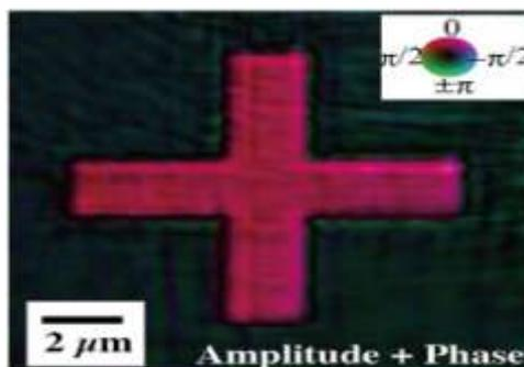
Figure 6. Complex amplitude image of crossed line pattern with the amplitude represented by brightness and the phase represented by hue. Reproduced from [10]. Copyright ©2013 The Japan Society of Applied Physics. All rights reserved.
