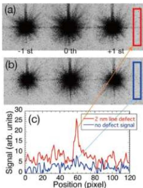
Figure 10. (a), (b) Observed diffraction patterns from an 88 nm L/S pattern, and (c) spatial profile of defects signal. Reproduced from [25]. Copyright © 2012 The Japan Society of Applied Physics. All rights reserved.
