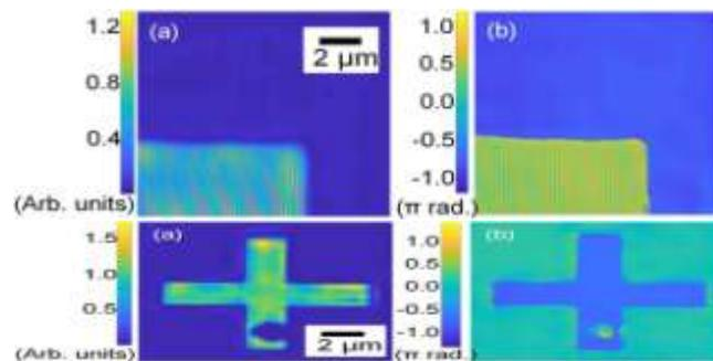
Figure 18. Reconstructed results of the corner structure of the 88 nm L/S pattern in terms of (a) intensity and (b) phase. Adapted from [28]. Copyright © 2017 The Japan Society of Applied Physics. All rights reserved.
