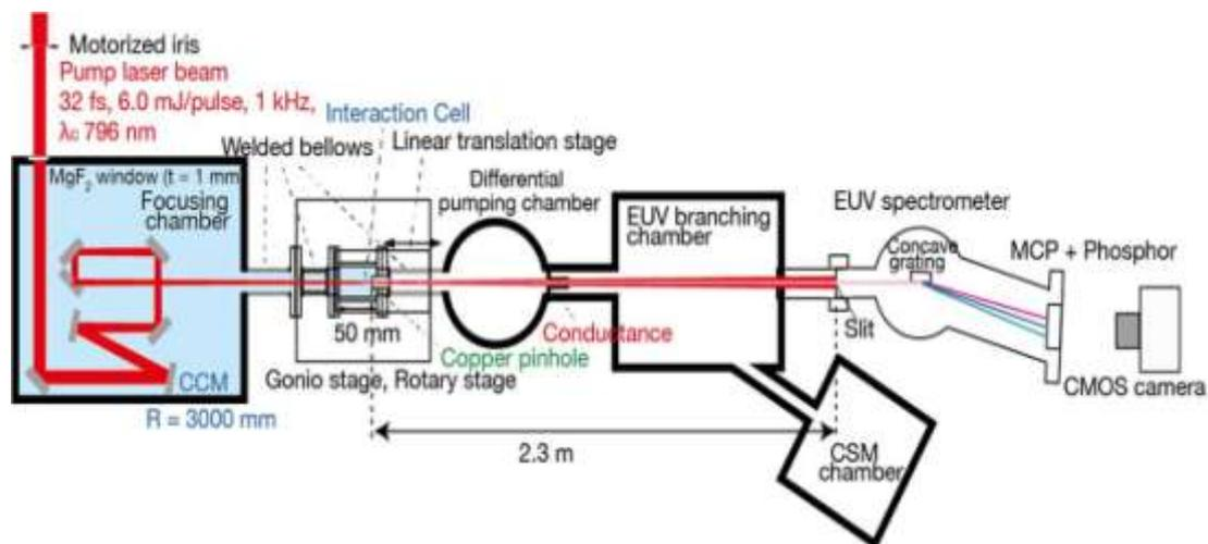
Figure 2. Experimental setup for high order harmonic generation.
