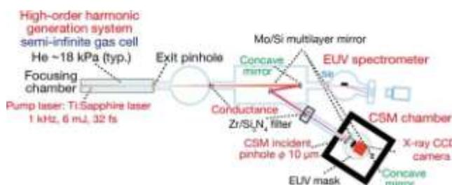
Figure 9. Optical double relay system for HHG-CSM system.
