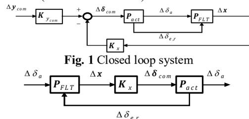
Fig. 2 Open loop system for aileron
