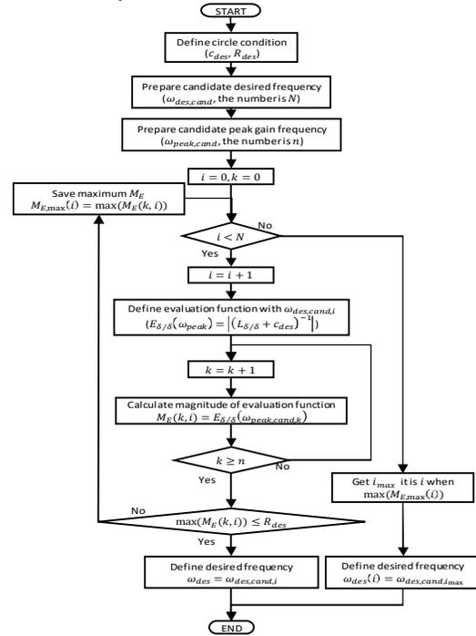
Fig. 3 Frequency Tuning algorithm
