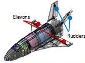
Fig. 4 WIRES rocket with control surfaces
