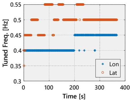
**Fig. 9** Tuning result of desired frequencies
