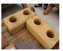
Picture 4. Soil Cement Block made with residual soil.
