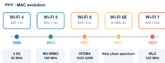
Fig. 1. Evolution from Wi-Fi 4 to Wi-Fi 7: successive gains in spatial multiplexing, multi-user efficiency, 6-GHz access, and multi-link coordination.
