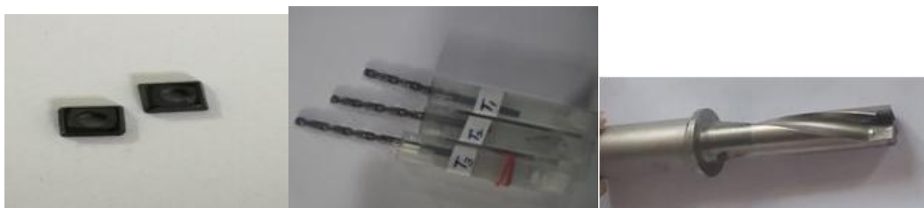
Figure 2. (a) Plain carbide inserts (b) Tungsten Carbide twist drill, & (c) U-drill
