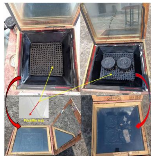
Fig 2. Solar box cooker with encapsulated PCM [4]
