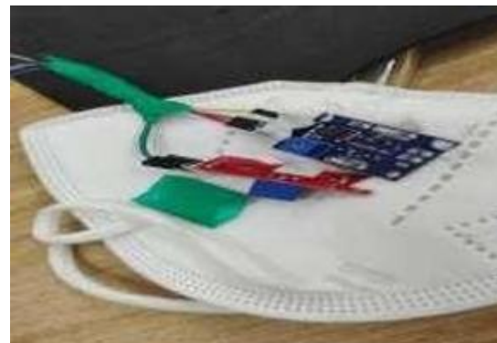
Fig4: Hardware Implementation of Sensor Embedded Intelligent Mask
