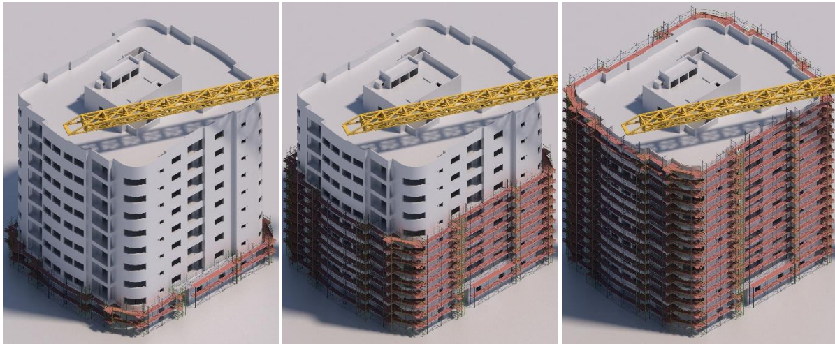
Figure 4. 4D sequencing of scaffolding construction illustrations, to show the erection and dismantling sequences (Illustrations by Author)
