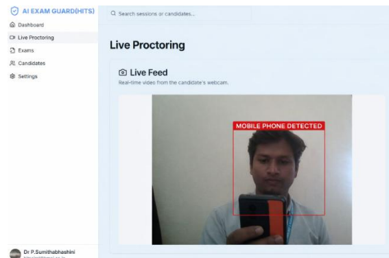
fig.7: sample outputs of audio-based surveillance and unauthorized device detection modules demonstrating real-time identification of suspicious acoustic activity and mobile phone usage.
