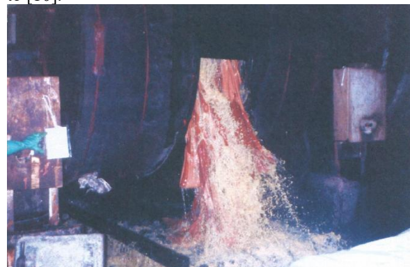
Fig. 7. Re-tanning occurring in a drum during the leather industrialization in a tannery in the Franca region. According to [12].
