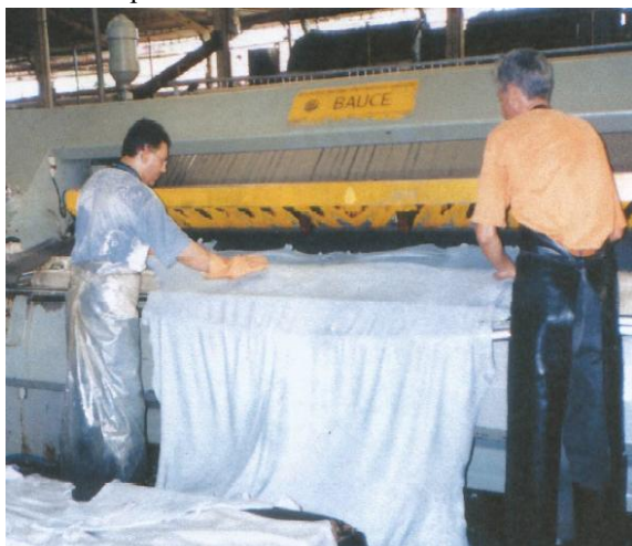
Fig. 4. Lowering of the “wet blue” leather in a tannery in the Franca region. According to [12].
