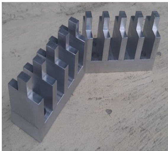
Fig: 2: Photograph of the 14 mm depth-cut heat sink model
