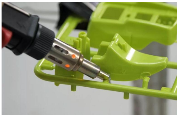
Figure 4. Soldering Iron Heated Gun for 3D Printing Parts Assembly
