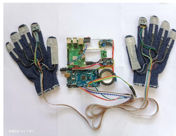
Fig. 3. Hardware implementation of the sign language-to-speech translation system.
