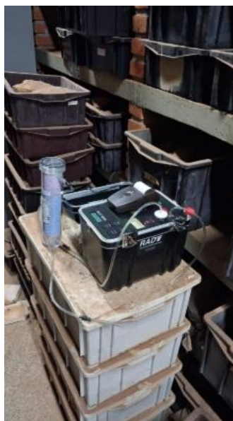
Fig. 6. Set up of RAD7 at litoteca (LIT), Geology Department, IGCE-UNESP-Rio Claro Campus.
