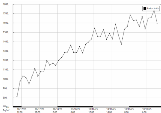
Fig. 13. Plotting of the radon emanation data of the granite sample (gravels). Duration of each measurement cycle = 1 hour.
