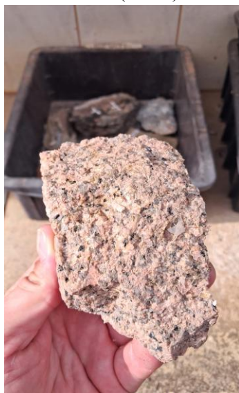
Fig. 7. Granite sample (GRA) used for radon exhalation experiments conducted at LABIDRO, Geology Department, IGCE-UNESP-Rio Claro Campus.
