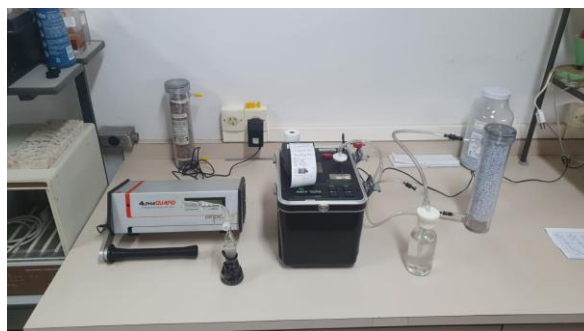
Fig. 5. Set up of RAD7 at LABIDRO (Isotopes and Hydrochemistry Laboratory) (LAB), Geology Department, IGCE-UNESP-Rio Claro Campus.
