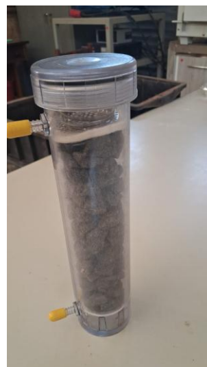
Fig. 8. Gravels of the granite sample (GRA) used for measurement of the radon exhalation conducted at LABIDRO, Geology Department, IGCE-UNESP-Rio Claro Campus.
