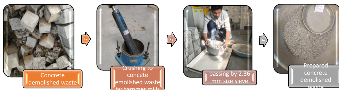
Fig-4. Process of concrete demolished waste (CDW)
