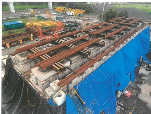
Placing of ISMB steel sections and rebar bundles on the FSLM Girder for completion of 90% test load
