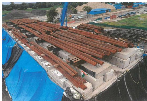
Placing of ISMB steel sections and rebar bundles on the FSLM Girder for completion of 90% test load
