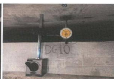
Position of Dial Gauges of foundation and Bearing regions for measurement of settlement and compression
