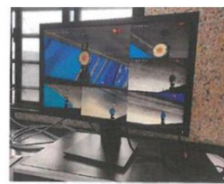
View of all Dial Gauge readings displayed in monitor through cameras placed in Respective position
