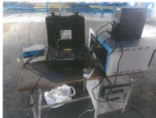
View of Data Logger where all the leads of LVDTs are connected
