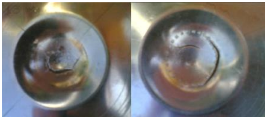
Figure (11): Models containing defects of large size.
