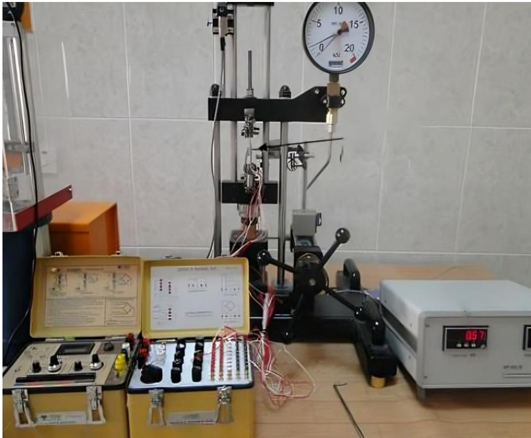
Fig (3) : Laboratory Tensile Testing Machine capacity ( 20 KN ) used for practical buckling test.
