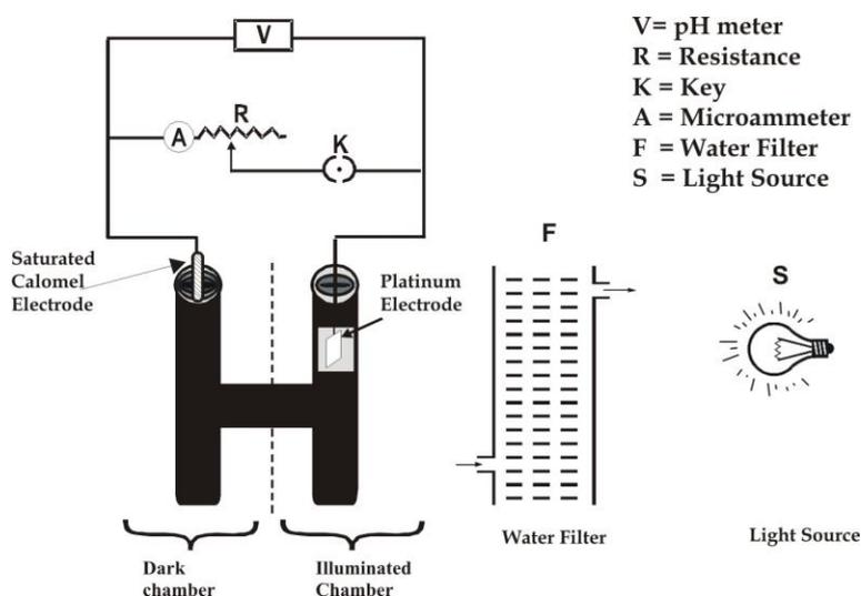
Fig. 1 : Photogalvanic cell set-up
