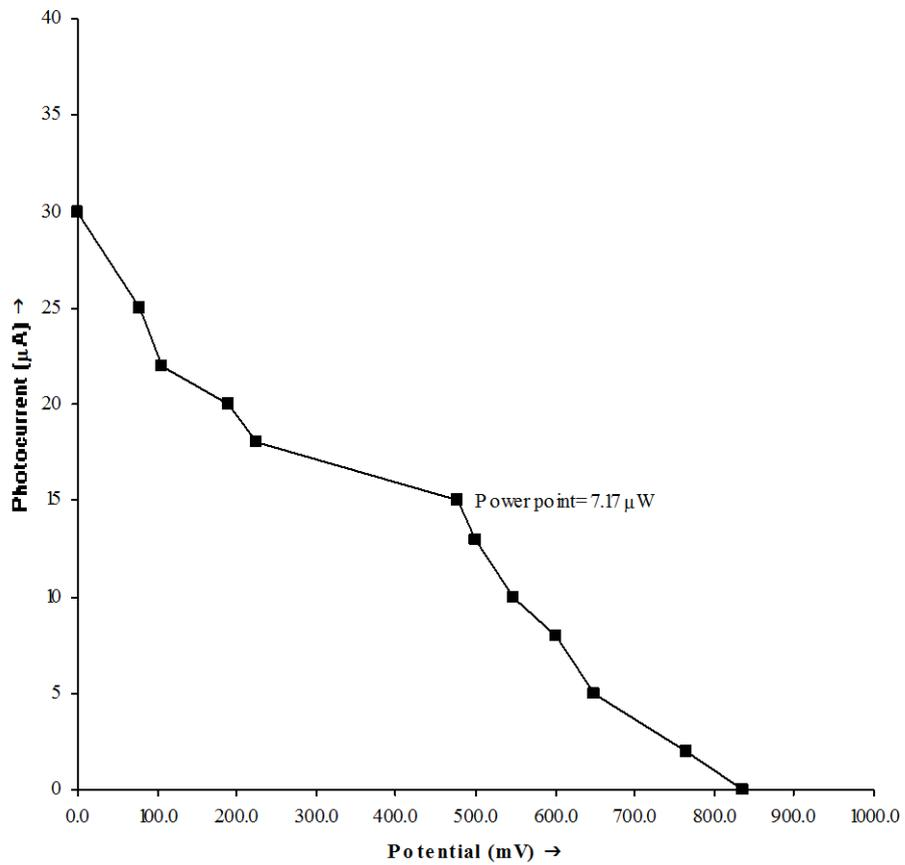
**Fig. 6. CURRENT-VOLTAGE (i-V) CURVE OF THE CELL**
