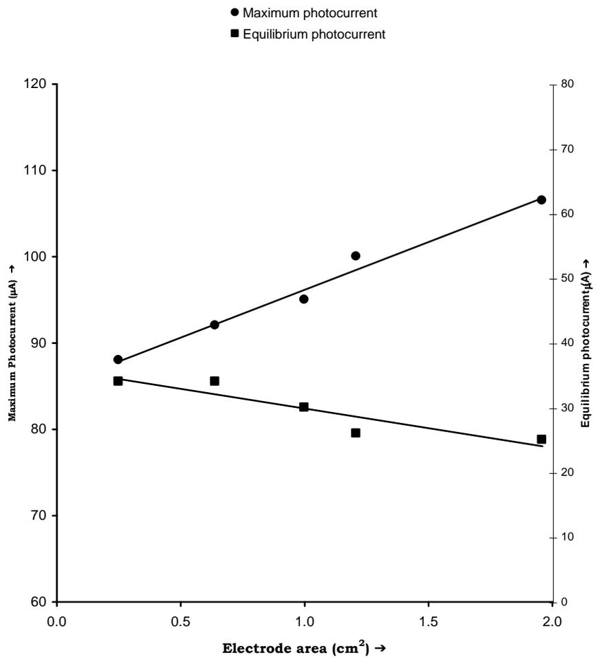
**Fig. 5. VARIATION OF CURRENT PARAMETERS WITH ELECTRODE AREA**
