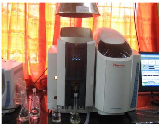
Fig 2. Photograph of Atomic absorption spectrophotometer
