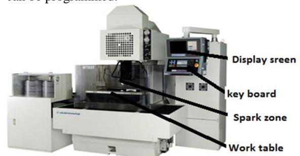
Fig. 2. Joemars WT-655 CNC Wire cut EDM
