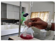
Fig.1 hardness test
