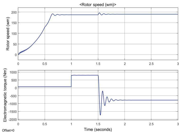
Figure 8 speed-torque output of classic IM for varying load torque input
