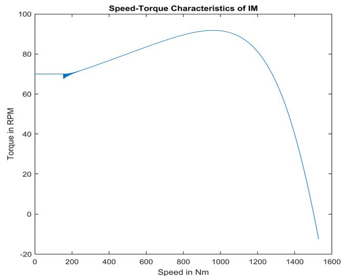
Figure 2. Speed-torque characteristics of IM
