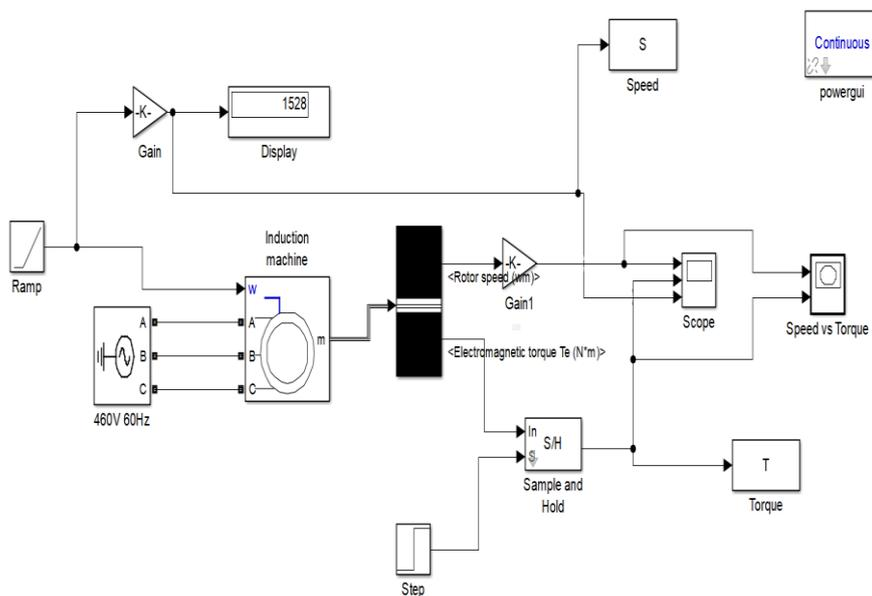
Figure 1 Simulation model of IM
