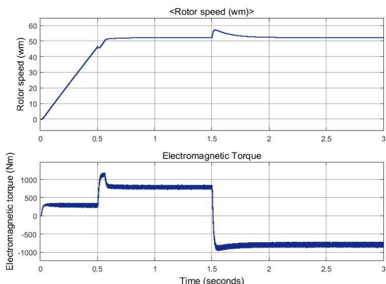
Figure 9 speed-torque output of DTC-IM for varying load torque input
