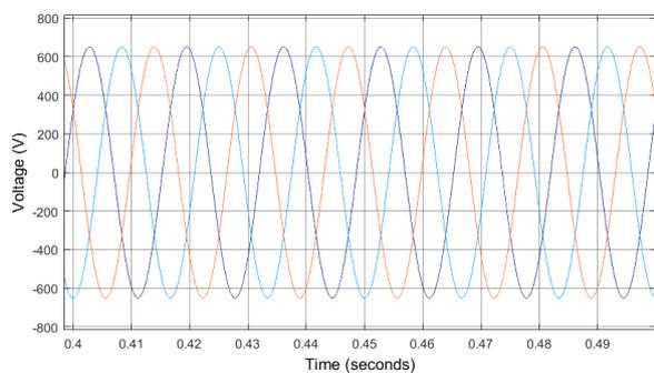
Figure 12 three phase source voltage input to the IM
