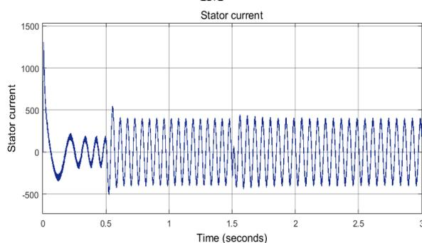
Figure 11 Stator current for phase 'a' in case of DTC-IM
