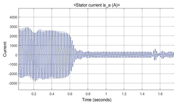
Figure 10 Stator current for phase 'a' in case of classic IM
