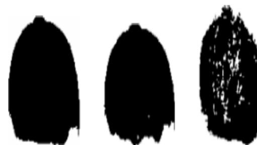
(g) Binary image on red band (T = 160). (h) Binary image on green band (T = 150). (i) Binary image on blue band (T = 80).
