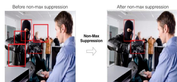
Fig 7. The process of non-max suppression is performed.
