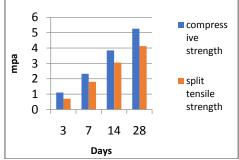
Compressive strength and split tensile strength of ECA :
