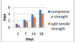
Compressive strength and split tensile strength of foam concrete :
