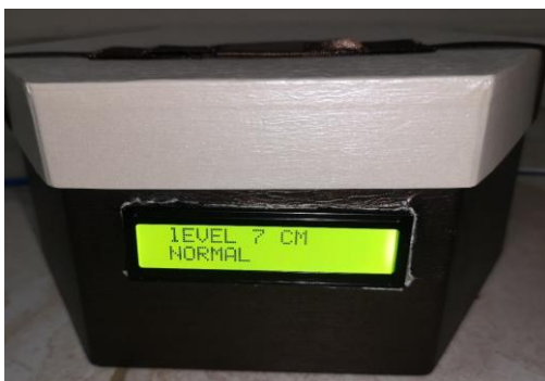
Fig.9: Normal level of the liquid in the I2C LED
