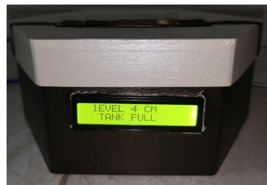
Fig.12: High level of the liquid in the I2C LED display
