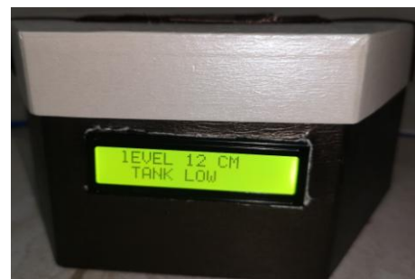
Fig. 6: Low level of the liquid in the I2C LED display
