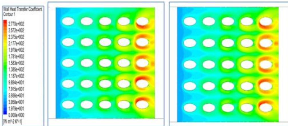
Fig 3.3: BC [1] & [2]  $HTC_w$  for  $Re = 30,000$  at lower end wall
