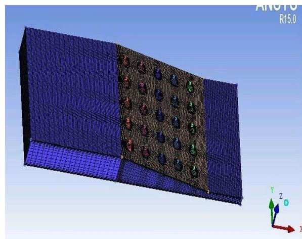
Fig 2.1: Elliptical Pinfin model and O-grid Meshed elliptical Model
