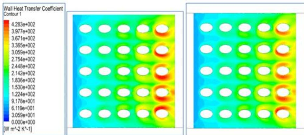
Fig 3.5: BC [1] & [2]  $HTC_w$  for  $Re = 50,000$  at lower end wall
