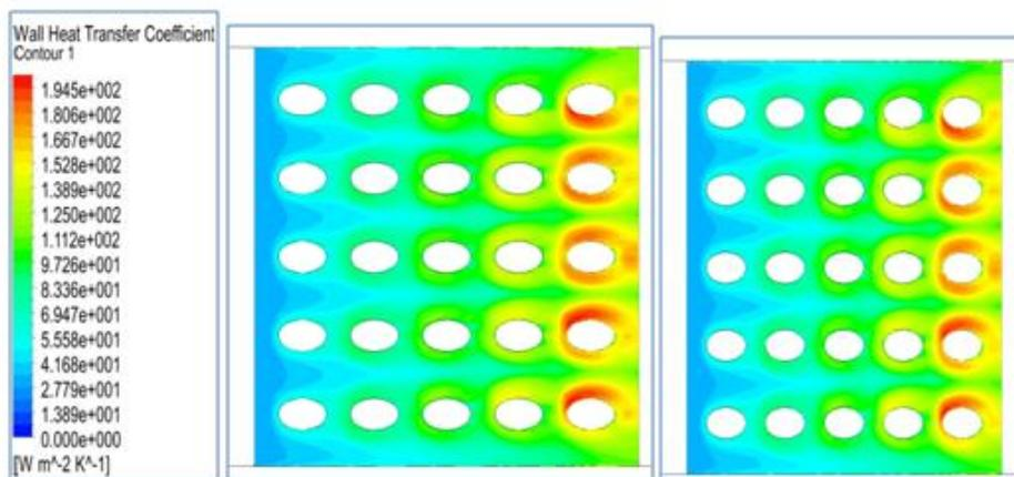
Fig 3.2: BC [1] & [2] for  $Re = 20,000$   $HTC_w$  at lower end wall
