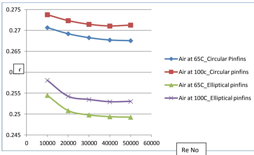
**Graph 1.1:** Comparison of coefficient of friction for BC [1] and [2] for pinfin
