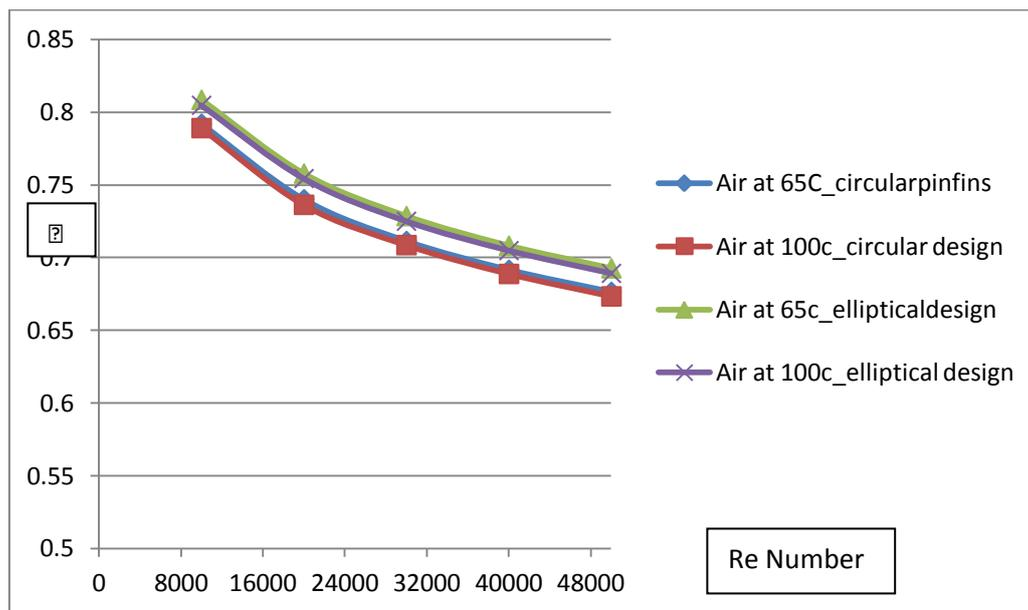
**Graph 1.2:** Comparison of coefficient of friction for BC [1] and [2] for pinfin
