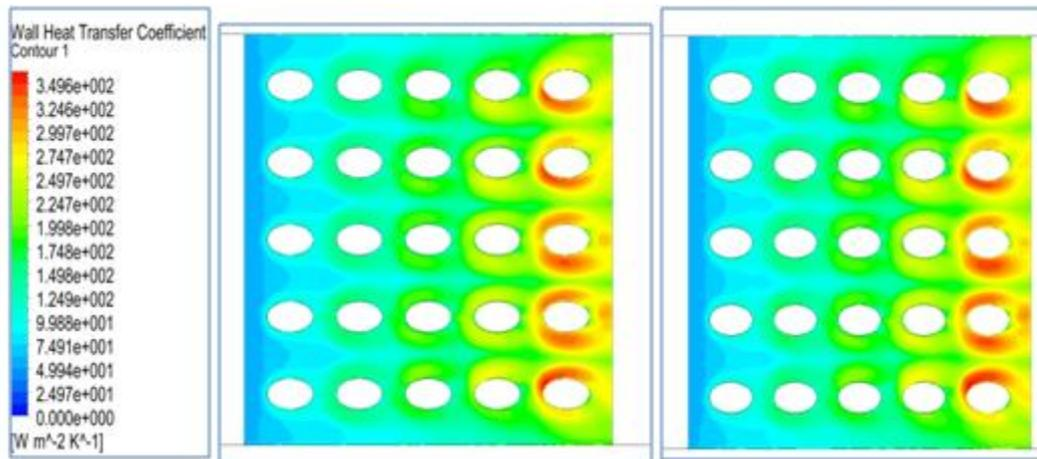
Fig 3.4: BC [1] & [2]  $HTC_w$  for  $Re = 40,000$  at lower end wall
