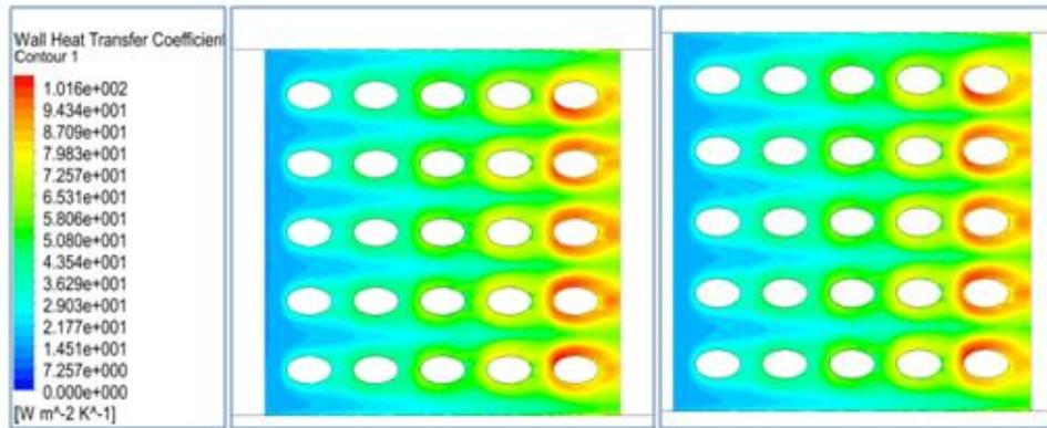
Fig 3.1: BC [1] & [2]  $HTC_w$  for  $Re = 10,000$  at lower end wall
