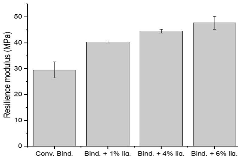
**Figure 6:** resilience module of conventional ligand and ligand modified with lignin.
