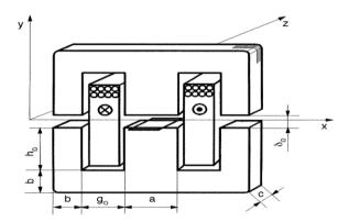
Figure 3. The E-type contactor electromagnet
