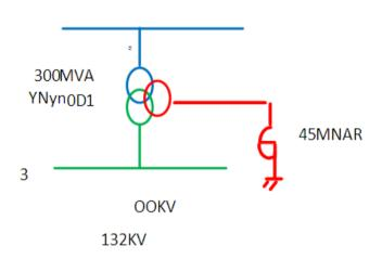
Figure 5 – Clock notation for **YNyn0D1** Transformer
