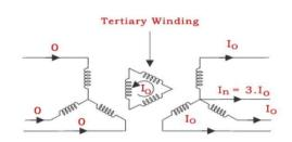
Diagram of Three Winding Transformer
