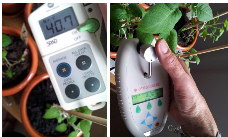
Fig. 1. Estimation the chlorophyll content of leaf portable device (SPAD 502 Chlorophyll Meter) (A) and the anthocyanin content at leaf (portable device ACM 200 plus, Antocianin Chlorophyll Meter) (B).
