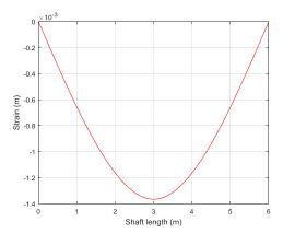
Figure 7. Strain distribution along the screw.
