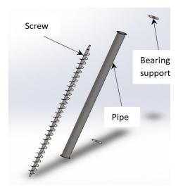
Figure. 1. Main components of an Archimedean screw.
