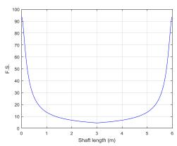
Figure 6. Safety factor distribution diagram along the screw.
