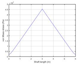
Figure 5. Stress distribution along the screw.
