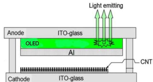
Figure 6: The schematic diagram of FE-OLED device.
