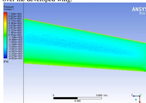
Fig. 15 Pressure distribution over the surface of the wing
