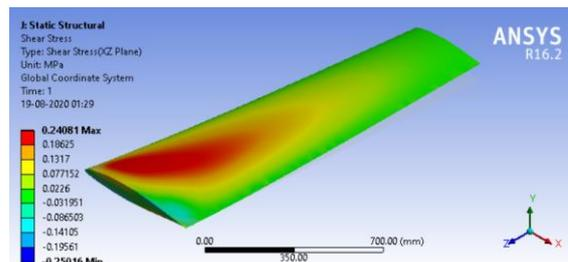
Fig. 13 Shear stress along the upper surface
