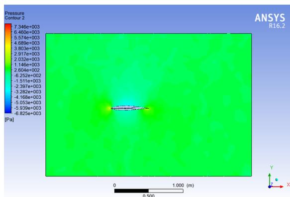
Fig. 16 Pressure distribution around the airfoil
