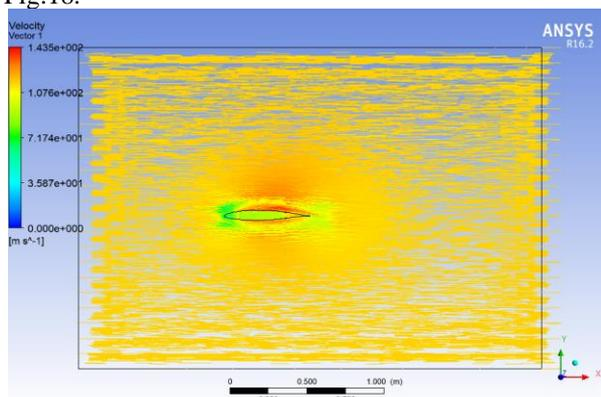
Fig. 17 Velocity contours around the airfoil
