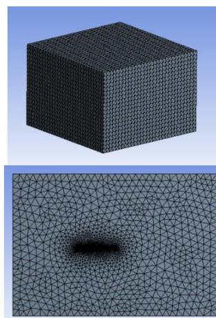
**Fig. 8&9** Mesh of the Fluid Model
