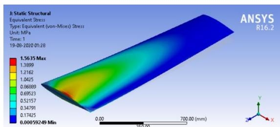
Fig. 12 Equivalent Stress
