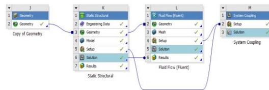
Fig. 9 ANSYS components Interaction
