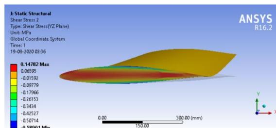
Fig. 14 Shear stress across the chord
