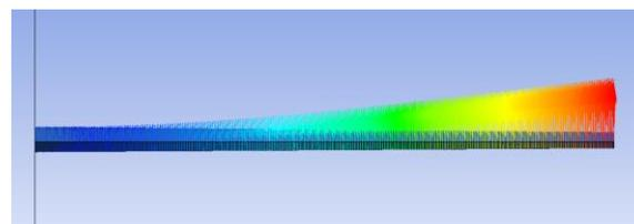
Fig. 19 Total Mesh displacement (Tip of the wing)
