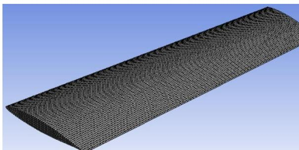
Fig. 5 Mesh of the model
