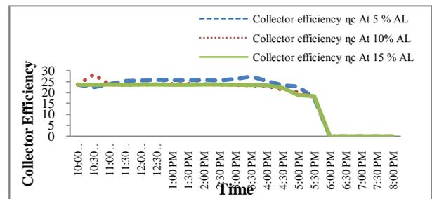
Fig.3 Variation of Collector efficiency w.r.t. to time of day .
