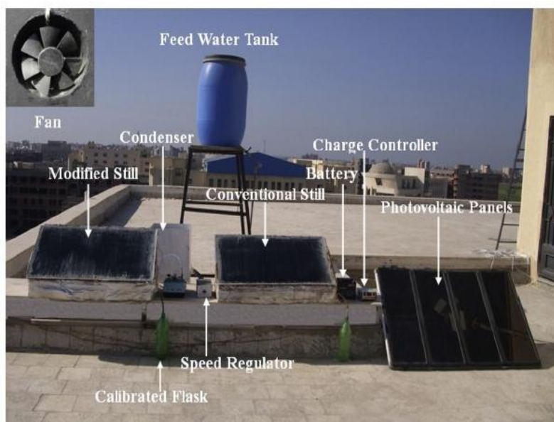
Fig.15 Photograph of the two conventional and modified solar stills ( Kabeel et al. [ 88 and 89] ).
