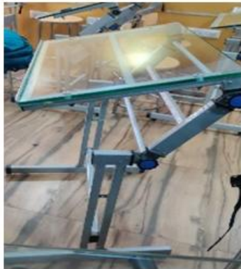
Figure 10: tempered glass board with easily adjustable screws and metal support. Source - References
