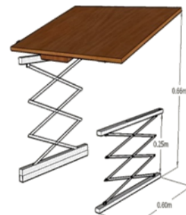
Figure 18: PORTABILITY The drafting table should be designed in such a way that, it can be easily detached and carried around. Source - References
