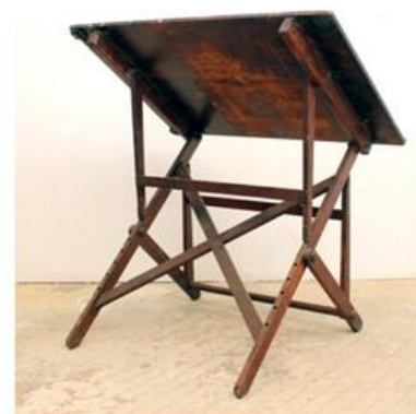
Figure 3: The adjustability was accomplished by adding dowels that could be placed into a series of drilled holes. Source - References
