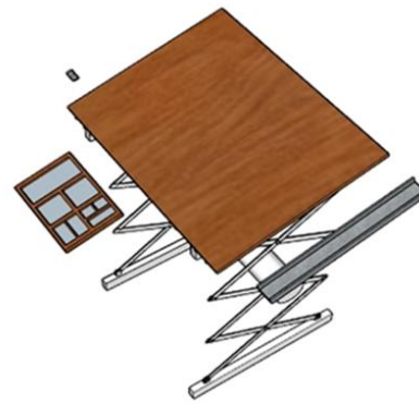
Figure 15: Exploded view of the proposed drafting table. Source - References
