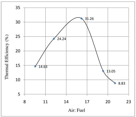
Fig 3 Variation of efficiency( $\eta$ ) with the variation of air fuel ratio
