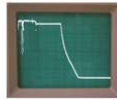
Fig (8) Collector-Emitter voltage
