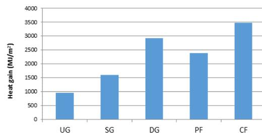
Figure 16 Useful Heat gain for different geometry of solar air heater
