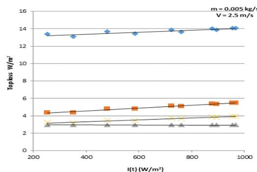
Figure 12 Top loss for different type of SAH
