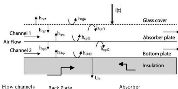
Fig 6 Cross sectional view and nomenclature
