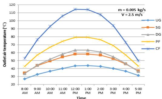
Fig. 10 Hourly variation of outlet temperature
