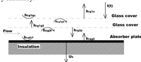
Fig.5 Cross sectional view and nomenclature
