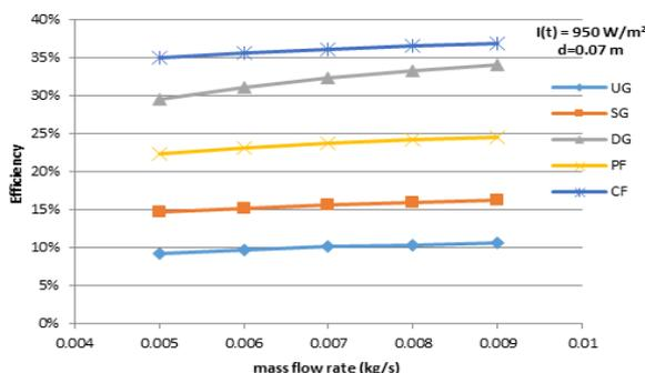
Fig 14 Efficiency variation with mass flow rate
