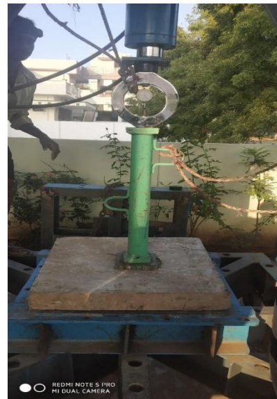
Figure 3. Punching test set up for simply support condition
