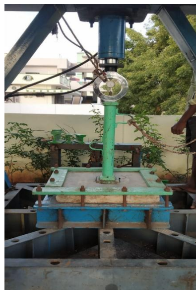
Figure 6. Punching test set up for fixed support
