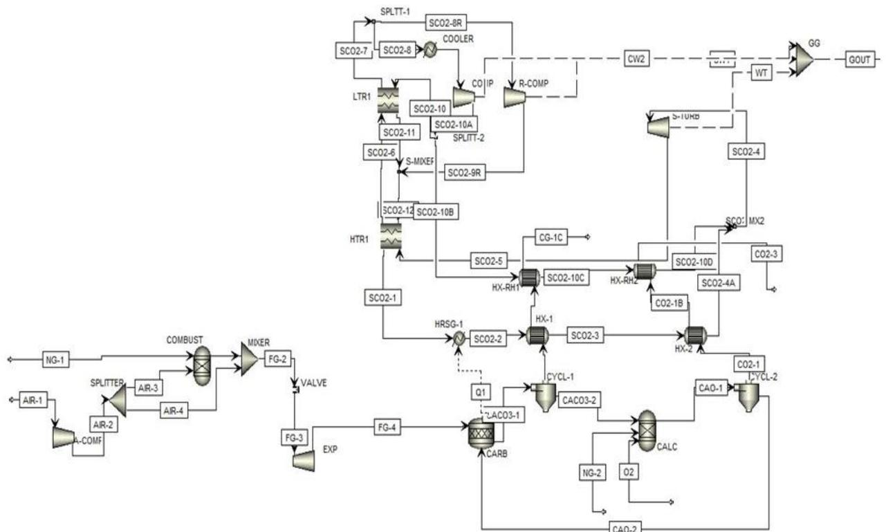
Fig. 1: Aspen plus Integrated NGCC plant with CaL
