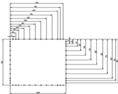
**Fig. 2:** Measuring locations of drill points for wall pressure measurement
