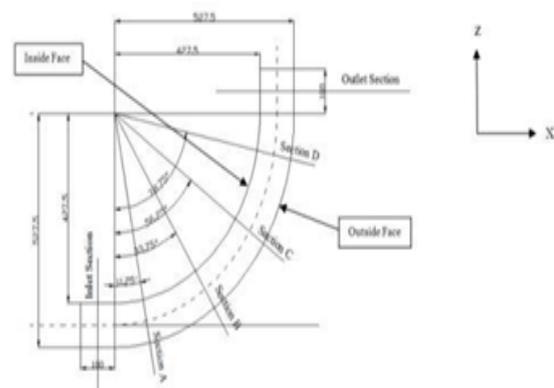
Fig. 1: Geometry of Curved Square C Shaped Duct
