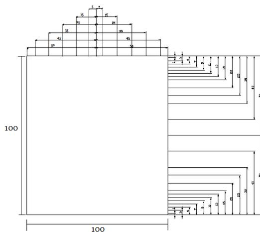
**Fig. 4:** Measuring locations of drill points for internal pressure measurement
