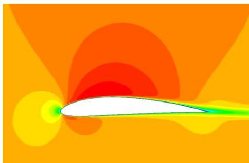
The graph of pressure contour shows a high pressure area below the airfoil due to the ground at close proximity. We can see vortex at the trailing edge of the airfoil which is due to the difference in pressure at the top and bottom of the airfoil. The low pressure area indicate the area of higher velocity. The leading edge experiences area of high pressure and is called the stagnation point.
