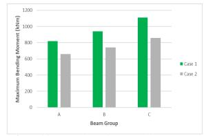
Figure 16: Comparison of Max Bending Moments in outer beams of bottom slab of Model B.
