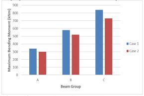
Figure 10: Comparison of Max Bending Moment in inner beams of Top Slab of Model A.
