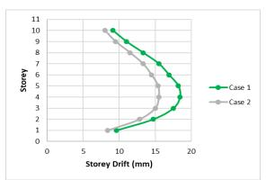
Figure 13: Comparison of Storey Drifts of Model B
