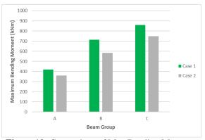
Figure 19: Comparison of Max Bending Moments in inner beams of Top Slab of Model B
