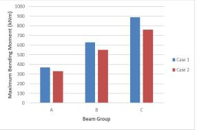
Figure 8: Comparison of Max Bending Moment in inner beams of bottom slab of Model A.
