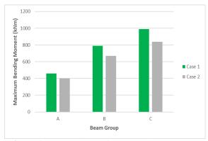
Figure 17: Comparison of Max Bending Moments in inner beams of bottom slab of Model B
