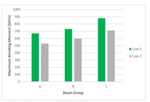
**Figure 18:** Comparison of Max Bending Moments in outer beams of Top Slab of Model B.
