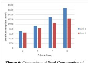
Figure 6: Comparison of Steel Consumption of Model A
