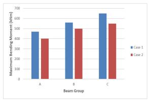
Figure 9: Comparison of Max Bending Moment in outer beams of Top Slab of Model A
