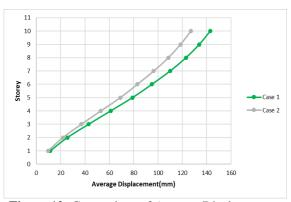
Figure 12: Comparison of Average Displacements of Model B
